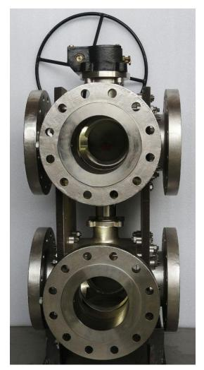
Rajeev & Company is proud to announce the arrival of their latest product KAVAATA 6 Way Ball Valve. This product is designed for Duplex Filters to achieve smooth changeover between the filters. The product shown in the picture is a 6" 6 Way Class 300# ASTM A351 Gr CF8M/ SS316 ball valve with gear operator.
